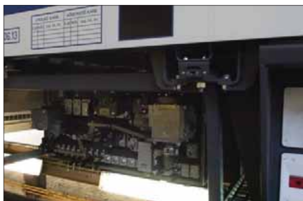
2. ábra: Fékonténer a BRT698- as fékpanellel Abb. 2: Bremscontainer mit Bremspaneel BRT698 Fig 2. Brake container with type BRT698 brake panel.
